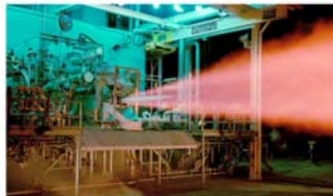
Source: EOP, Inc. http://www.eop.com/pressroom/050905a10 The photo shows a ground test of a Space Shuttle main engine liquid oxygen (LOX) turbo pump. Testing is critical to assure that the component can deliver the required performance. The LOX turbo pump for each of the Shuttle's main engines produces 26,800 horsepower of pumping action and spins at 23,700 revolutions per minute. Each of the corresponding fuel turbo pumps delivers 76,000 hp – the power of 28 locomotives – and spins at an even more incredible 36,200 rpm.
